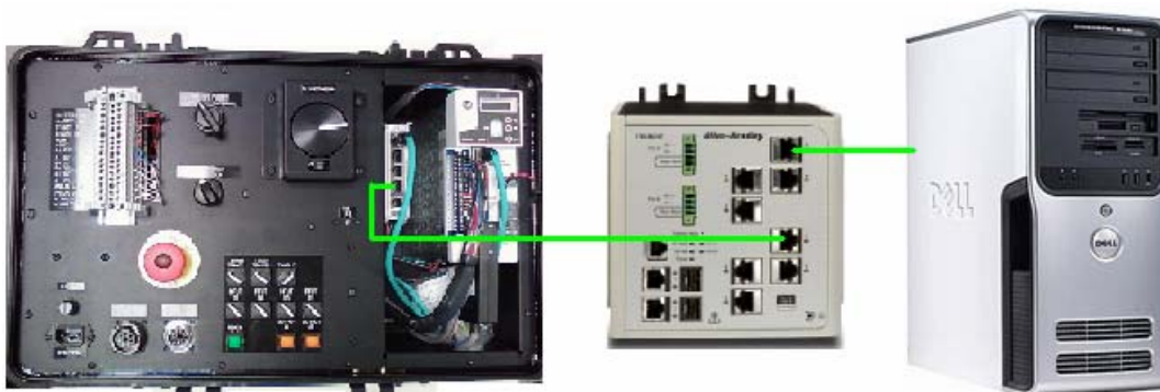
Typical Ethernet Layout (a switch is shown, but is not required)
